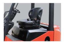
Operator Presence System (OPS) — When operator is not in seat, the hydraulic lift and tilt controls automatically lock out and traveling is disabled.
