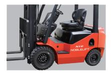
Heavy-duty steel chassis, axles, mast and overhead guard deliver high strength and stability for high lifting heights and heavy loads.
