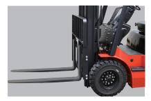
Intelligent buffering effectively protects the ground and cargo from damage while forks descend to the ground.
