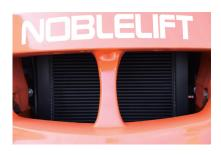
Radiator's plate fin heat dissipation system keeps engine running reliably, even in the most demanding applications.
