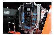
Durable controller that integrates all electrical components is protected from temperature, water and vibration.
